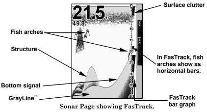
When the boat is not moving, fish signals are long, drawn out lines on a normal chart display. FasTrack converts the graph to a vertical bar graph that, with practice, is useful for stationary fishing.
